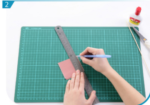
Use a pen whose ink has dried out, or a tracer, to trace lines first.
